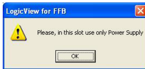
Fig 3. 170 – Error – Inserting modules in the Rack Z (1)
