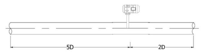
At flowmeter upst ream, there should be straight pipe no less than 5D and no less than 2D at flowmeter downstream. (D is the inner diameter of flowmeter)
