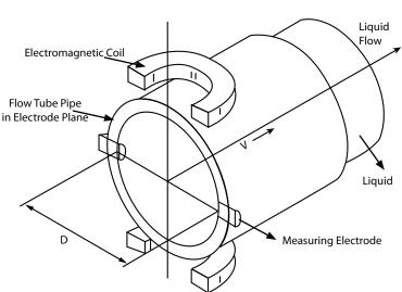
The induced voltage is not affected by the physical properties of the liquid like temperature, viscosity, pressure, density and conductivity, as long as the conductivity of the measured liquid is above a minimum threshold.
