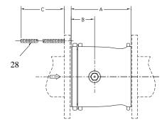
Figure 4. Required clearances for installation of design CVS V-100 Ball Valve Body
