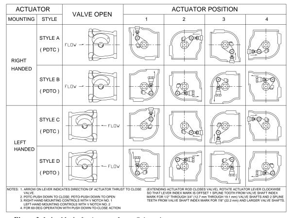
Figure 3. Index Marks for Actuator Lever Orientation
