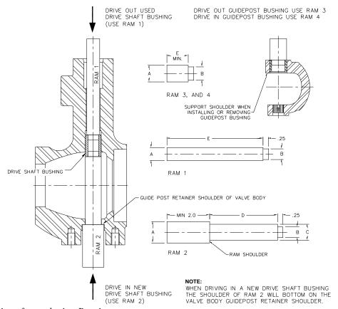
Figure 5. Ram Dimensions for replacing Bearings
