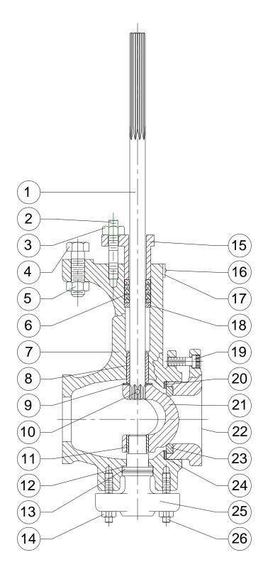
Figure 12. Typical Cross Section of 2-8 inch Design CVS V-100 Ball Valve
