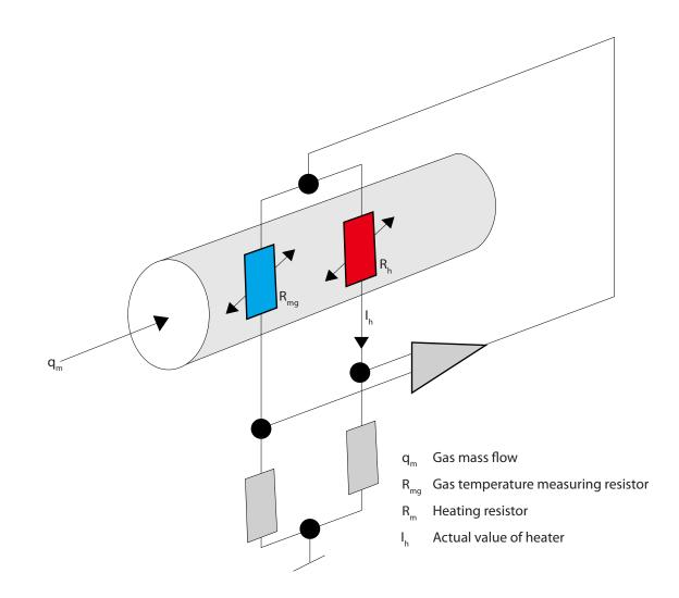
Tek-Thermal 1700B Thermal Mass Flowmeter design is based on constant power measuring method, thus the RTD is heated on a consistent power and will be more durable and stable. Due to that, Tek-Thermal 1700B has less problem of zero-off which may cause a function failure of RTD due to overheating the term.
