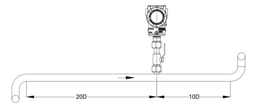
Installation when valves or pressure controller or any other device may cause turbulence in the upstream or downstream of the flowmeter
