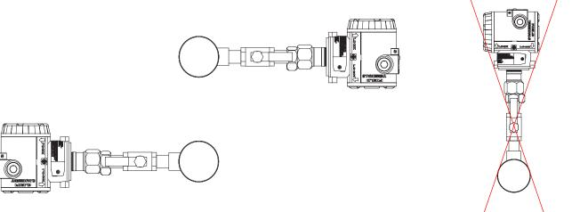
On the side of the pipe. Not recommended to install the meter above the pipeline
